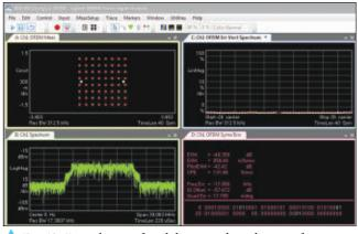
▲ Fig. 10 Key indicator of modulation quality when interferer is dormant.
