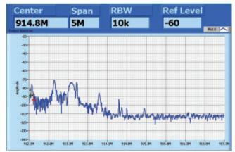
▲ Fig. 11 Second harmonic distortion with preselector module included.
