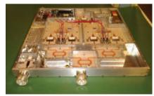
▲ Fig. 3 800 W S-Band SSPA module assembly.
