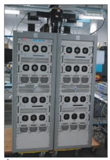
Fig. 5 10 kW S-Band phase combined amplifier system.
