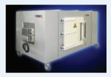
everberation chambers (RVC) are modern EMC test environments that provide an alternative to semi or full anechoic rooms (SAR/FAR), open area test sites (OATS) or Gigahertz Transverse Electromagnetic (GTEM) cells. The new RVC XS and 2XS models expand Teseq's extensive chamber portfolio.
