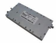
from damage due to any out of spec DC voltage conditions that may be applied. Its rugged construction guarantees fault-free operation in the most extreme environments. It features 5 W output power, 37 dB linear gain, rise and fall time < 1 usec, +12 V DC, 1.8 amps at 100 percent duty cycle, and is 5"  $\times$  2.5"  $\times$  0.51".
